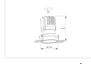
Beam Angle 38° Light Distribution Flood LED Type COB LED Light Source Osram SOLERIQ S 19 Start Time Instant Driver Stand Alone (included) **Operating Position** Non - Swiveling Type On-Off / Triac / 0-10 V Dimmina Construction Round Mounting Type Recessed Single Head Heads **Body Material** Aluminium Die cast Finish Black 4" Height 6-1/2" Diameter Cut Out 3" Darklight Technology Black, Silver Optics
